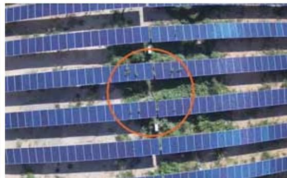
**Figure 3. Vegetation over the modules detected with aerial inspections applying two different techniques: aIRT (left) and aerial visual inspection (right)**
