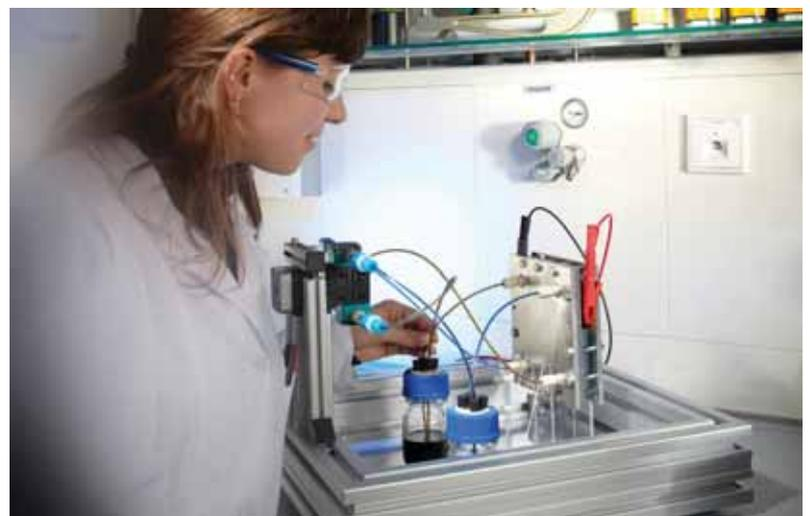
**Figure 3. Vanadium redox flow laboratory test cell setup**
