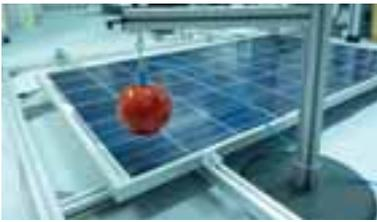
Figure 2. Set-up for Test 4 – tool drop test.
