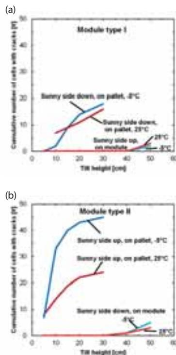
**Figure 9. Cumulative cell breakage as a function of the tipping height of the short edge of (a) module type I and (b) module type II. The results for Test 5 (sunny-side down) and Test 6 (sunny-side up) at +25°C and -5°C are shown.**
