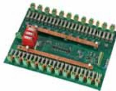
bloxx provides current measurements typically 10 times more accurately and is not susceptible to temperature variance. In addition, string voltage (up to 1,000V) and DC power on every string
