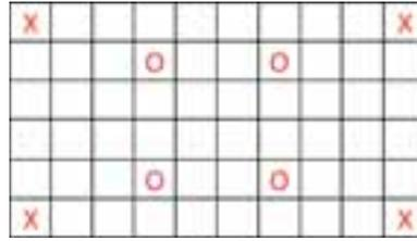
Figure 3. Pattern of the positions chosen for the drop test. The square grid indicates the cells in the module (x = corner drop locations; o = centre drop locations).
