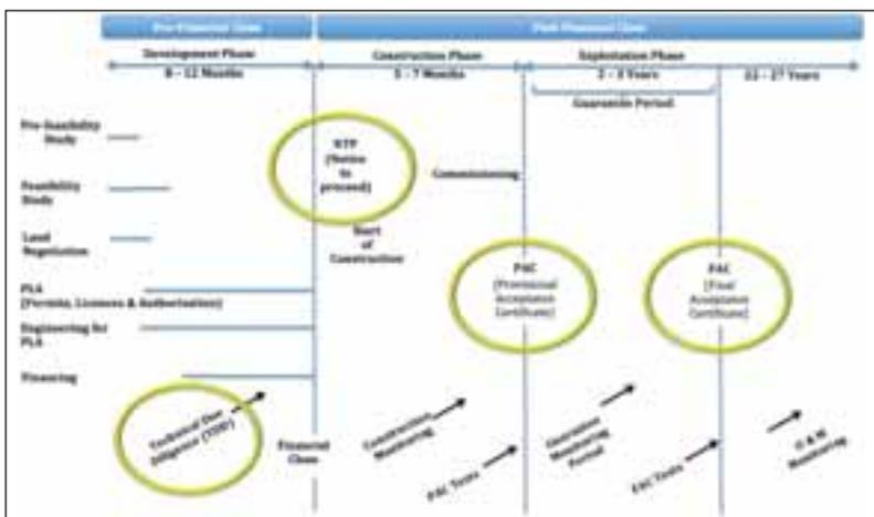
**Figure 2. Stages of a typical utility-scale PV plant.**
