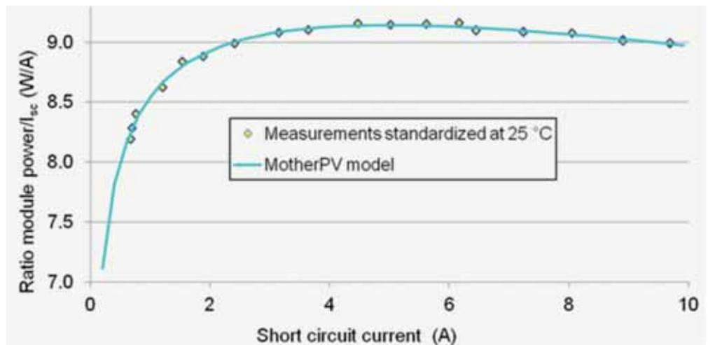
Figure 9. Mother-PV method: measurement and modelling of the ratio of P<sub>max</sub>/I<sub>sc</sub> versus I<sub>sc</sub> (at 25°C). Plotted against the short circuit current I<sub>sc</sub> that serves as a self-reference for irradiance
