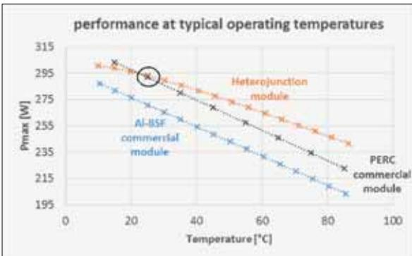
Figure 5.  $P_{max}$  under one sun versus temperature for SHJ, PERC and AI-BSF modules measured on Eternalsun Spire labflasher with temperature box. The black circle points to the performance of SHJ and PERC at STC conditions ( $25^{\circ}C$ )
