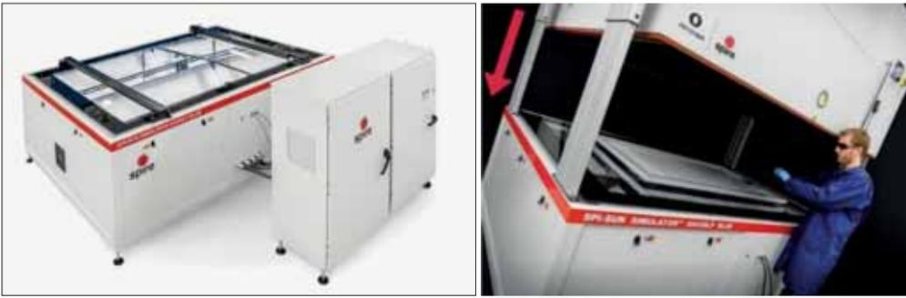
Figure 3. Left: SPI-SUN 5600 SLP table top simulator from Eternalsun Spire. Right: the same setup with an added temperature control box on top, ready for single-sided bifacial measurements
