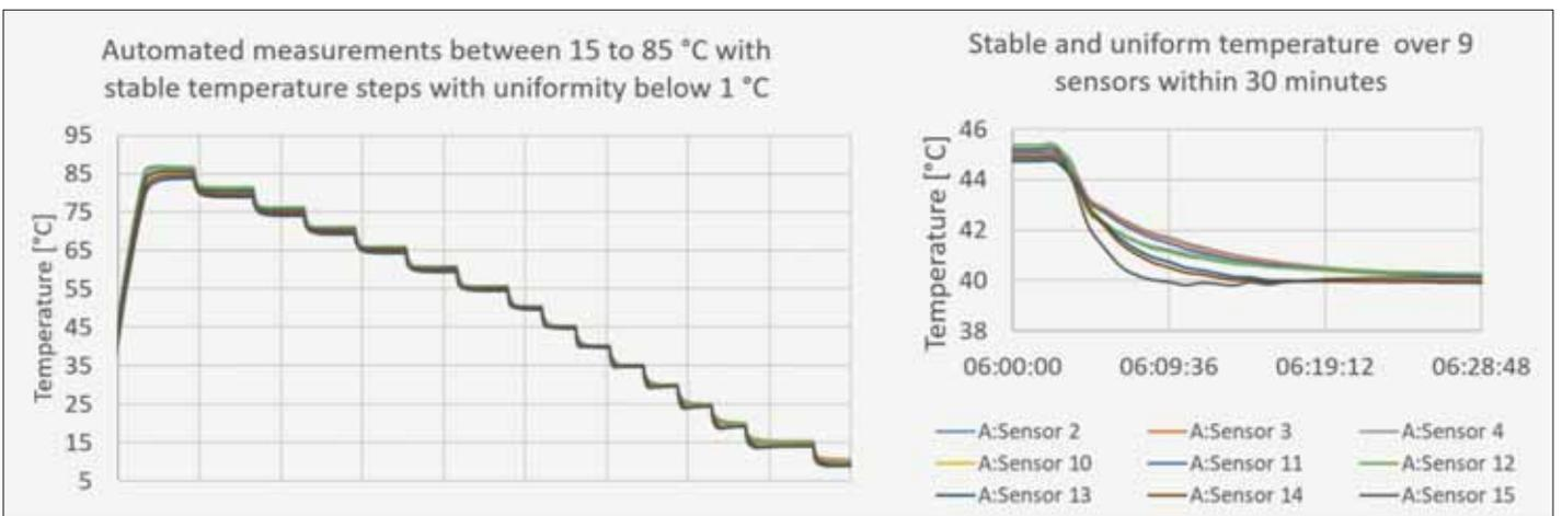
Figure 6. Temperature of the PV module on nine points across the module versus time during the  $P_{max}$  versus temperature test shown in Figure 5. Note that the temperature is stabilised for accurate  $P_{max}$  measurements. Test performed on the Eternalsun Spire setup shown in Figure 3
