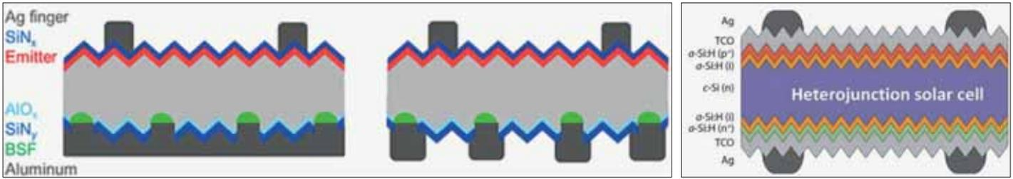
Figure 7. Layout of monofacial PERC (left) and bifacial PERC+ cell (middle) and heterojunction cell (right)
