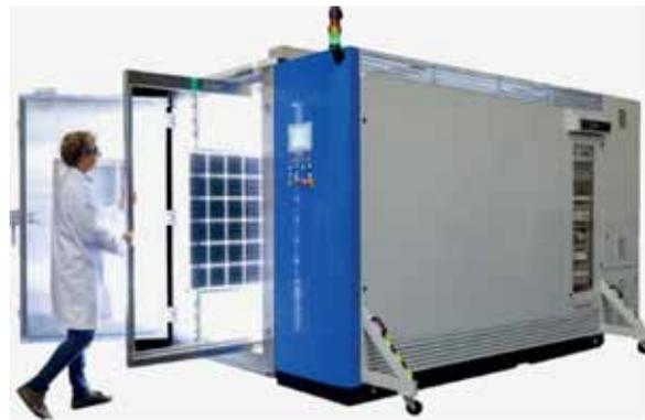
**Figure 10. Climate Chamber Solar Simulator (CCSS), capable of performing accelerated temperature, irradiance and humidity test on modules of different PV technologies**
