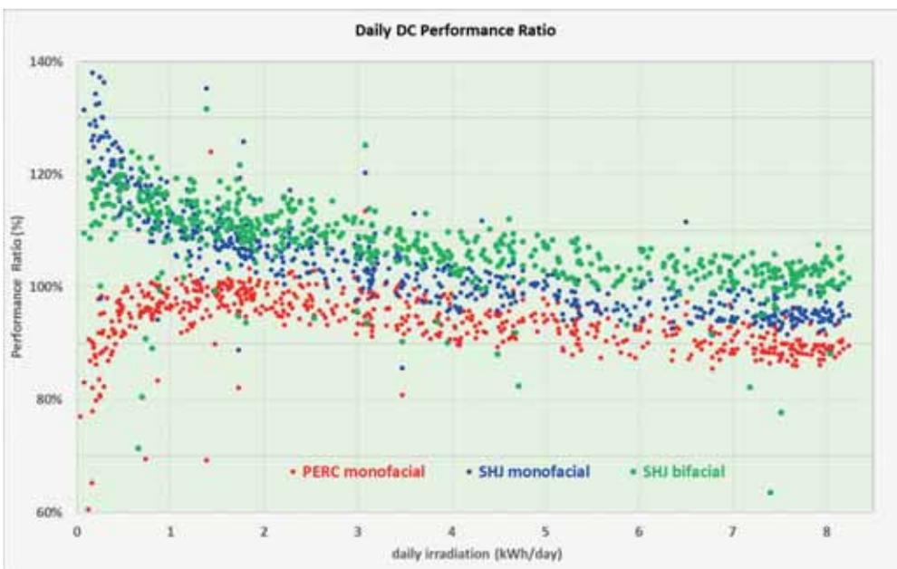
**Figure 13. Outdoor monitoring over 2016-2018 of the average daily performance ratio as a function of daily irradiance. Bifacial SHJ system in green**
