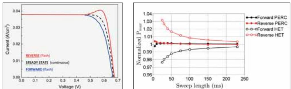
Figure 2. Left: IV curves for forward (blue) and reverse (red) short pulse sweeps compared to a steady-state IV measurement. Right:  $P_{max}$  performance measurement for PERC and SHJ modules as a function of pulse length on an Eternalsun Spire long-pulse solar simulator. Measurements converge at pulse lengths above 200ms, not attainable for conventional flash solar simulators
