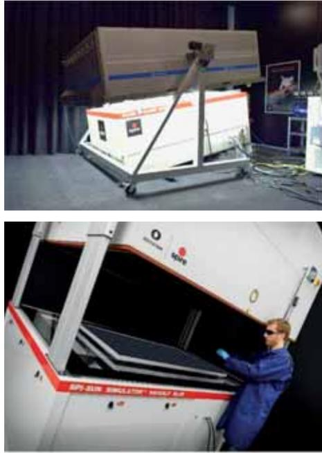
Figure 8. Two bifacial characterisation methods of bifacial with reduced footprint, tested by Eternalsun Spire. The single-side setup is commercially available and already installed around the world
