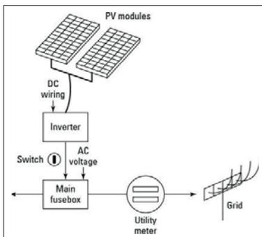
**Figure 2. Simple PV system block diagram**
