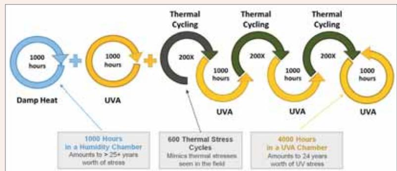
**Figure 3. Module Accelerated Sequential Testing, where repeated sequential stress mimics field degradation not detected by single tests and current industry standards.**
