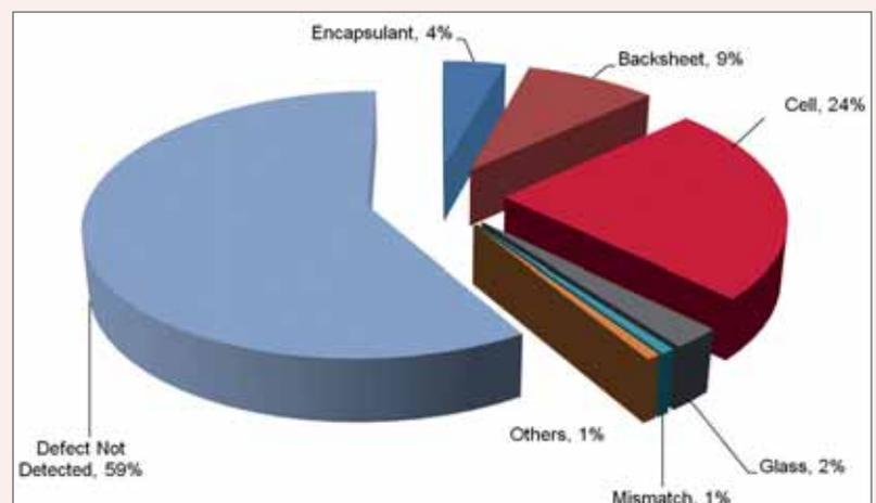
Figure 1. 41% of inspected modules exhibited some visual defect. Source: DuPont global field module survey of 71 installations (912,000 modules at 203MW) in North America, Europe and Asia Pacific.
