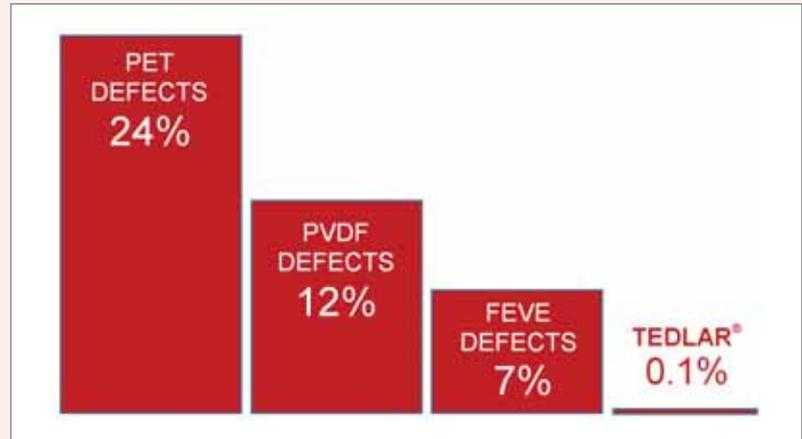
**Figure 2. Defect Rate by Backsheet Type.** Only 0.1% of the DuPont™ Tedlar® based backsheets showed defects. PET = Polyethylene terephthalate. PVDF = Polyvinylidene fluoride. FEVE = Fluoroethylene vinyl ether. Tedlar® PVF = Polyvinyl fluoride film.
