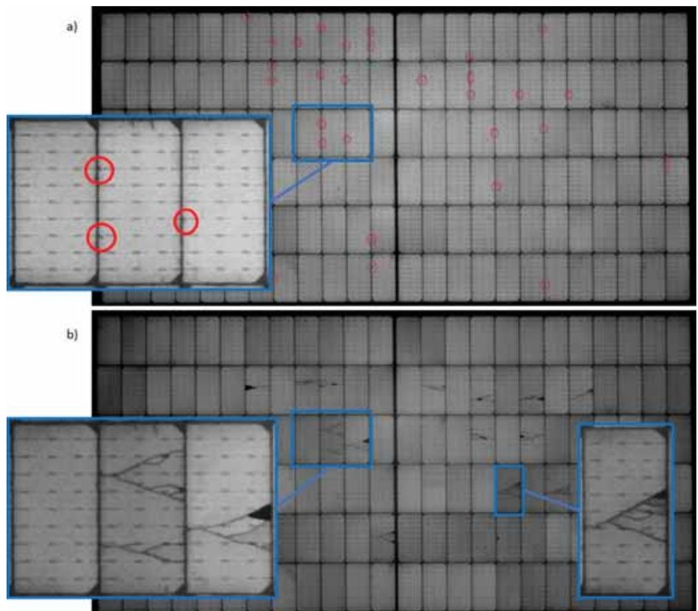
**Figure 1. a)** EL image of a PV module presenting cross-crack defects at cells' edges recorded by Enertis during batch acceptance testing; **b)** EL image after DML test (1000 cycles, 1000 Pa).
