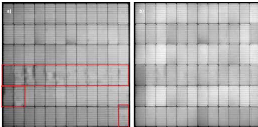
**Figure 2.** EL pictures of the same half-cut cell PV module (left side section) revealing marked defects associated to weak busbar soldering processes; a) registered by Enertis laboratory (10.6A polarisation DC current, CCD sensor); b) El picture recorded by the manufacturer (6.1A polarisation DC current, CMOS sensor) for inline quality control.
