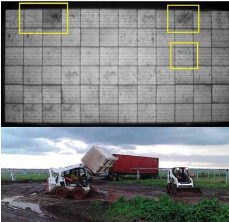
**Figure 4. Example of mishandling onsite. The cracked cells in the EL image were produced by the toes of the forklift during transport of boxes across the site, which packaging were, in turn, upgraded for future shipments.**
