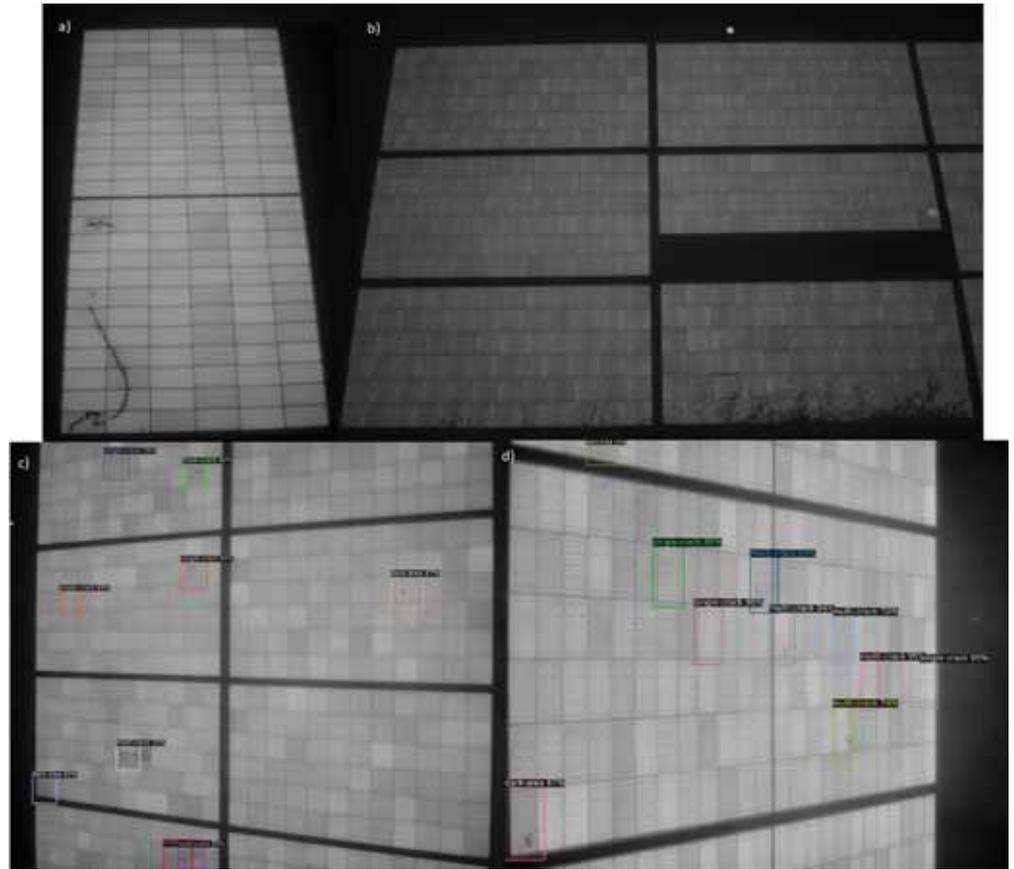
**Figure 5. Examples of EL defects found on different PV modules installed in different locations worldwide; a) critical extended linear defect derived from rear side's cell damaging (typically from backsheet scratching issues); b) manifest junction box issue (either faulty diode or connection) leading to cell substrating inactivity; c) and d) cell cracking defects and other minor issues accurately detected and categorised by Enertis EL software.**
