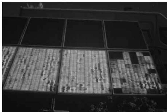
**Figure 8. Multiple defects found through EL in a PV plant affected by a massive flood issue. The EL inspection made possible an integrated diagnosis of the asset condition. Power and electrical insulation tests were also conducted, correlating data with EL outcomes. Serious degradations affecting power (disconnected cells, severe cracking defects) and safety issues (contacts corrosion) were eventually reported, defining subsequent actions to be triggered.**
