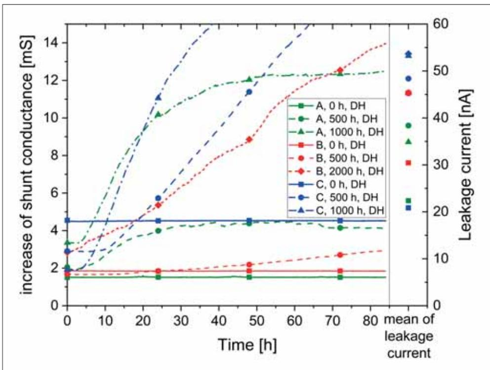
**Figure 5. PIDcon PID tests at mini modules after different durations of damp heat soaking exhibit a significant increase of the PID (shunting) susceptibility of modules due to increasing water content of the front EVA**
