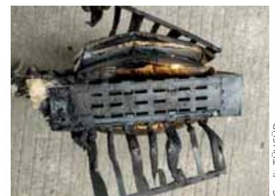
**Figure 5. A module of cells burns during external short-circuit test.**
