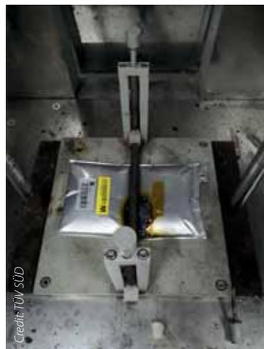
**Figure 4. Cell burning during impact test**
