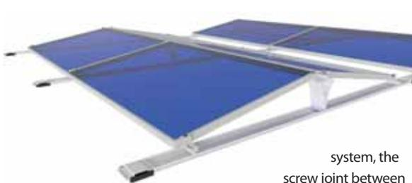
system, the screw joint between the rails and connectors does not need any nuts. The system requires just five main components and the standard Renusol module clamps, which makes mounting and storage simple. The maximum rail length is 2.3 m. Fewer components and shorter rails provide advantages for wholesalers, for installers, who can mount the rails quickly and easily,
